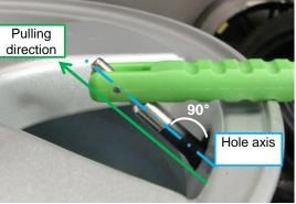
If the pulling direction is not correct or the valve is not rotated, the valve stem notches may damage the walls of the rim hole.
