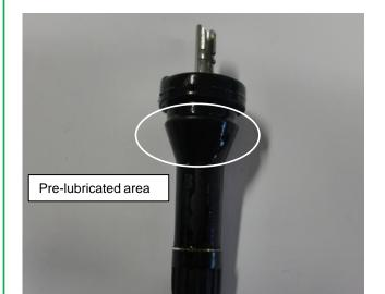
Do not install a valve without lubrication or fail to lubricate the conical section.
