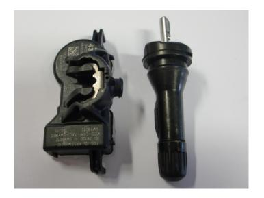
Do not install a valve that has a sensor attached as the sensor may be damaged
