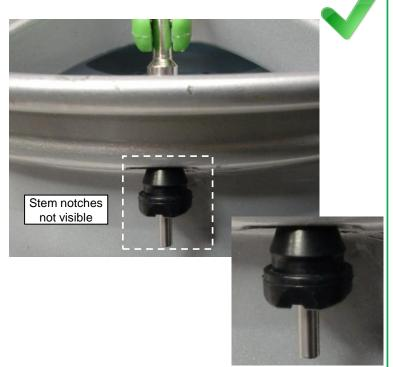
If the valve stem notches are visible, it is not possible to install the sensor.
