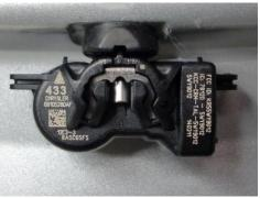
The sensor shall be firmly pushed to achieve the minimum possible gap. If needed press and hold the clip to unlock again and push
