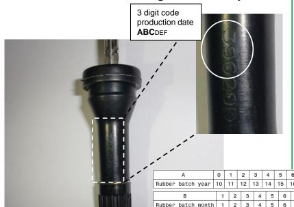
See table below to decode the valve production date from first three digits of valve marking.
