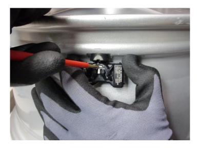
Do not try to remove the sensor from the valve stem without pressing the clip.
