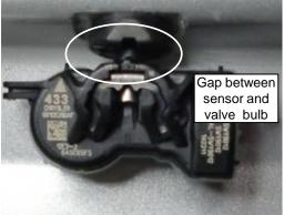
Do not apply excessive force to press the
