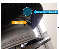
View from the rear-bottom of the mounting machine. As the sensor is at the right position (under the mounting head) it is not touched by the tire.
