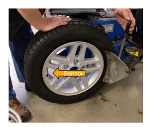
Don't position the bead breaker at the sensor position as it may be damaged
