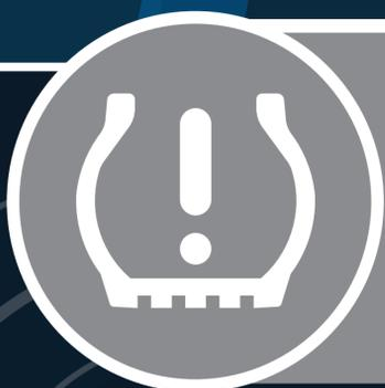
A TPMS warning light that stays on indicates **low tire pressure**. Check tire pressure and inflate as needed. If a tire is flat or going flat, change it immediately - **do not drive on it!**
