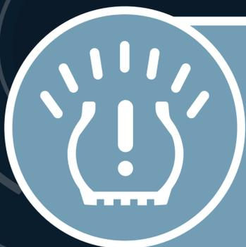
A TPMS warning light that flashes for 60-90 seconds, then stays on, indicates a system malfunction. **Seek professional service.**
