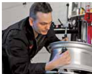
Hold sensor firmly in place while tightening hex nut.
