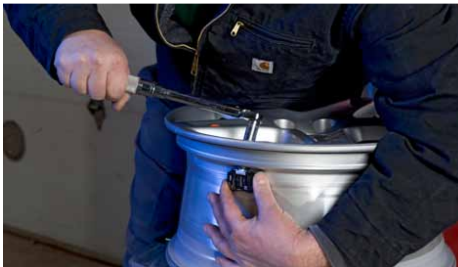
TPMS Sensor installation utilizing torque wrench.
