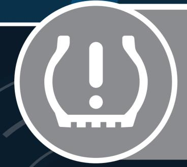
A TPMS warning light that stays on indicates low tire pressure. Check tire pressure and inflate as needed. If a tire is flat or going flat, change it immediately - do not drive on it!
