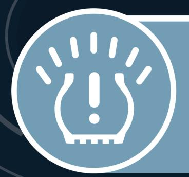
A TPMS warning light that flashes for 60-90 seconds, then stays on, indicates a system malfunction. Seek professional service.
